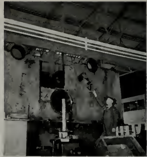
Arthur Tamberg, Bethlehem Machine Shop Supervisor, points to hole torn in Mobilube reduction gear casing by forepedo explosion.
